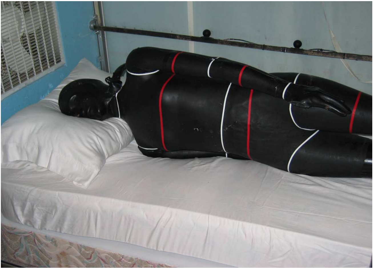
Figure 1. Nude manikin on mattress in environmental chamber.
